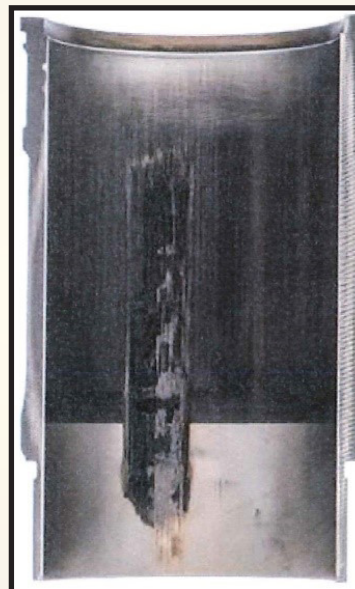
Severely scuffed liner after 47 hours
