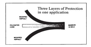
NOTE: See "How To Apply MIGHTYPLATE Products" Booklet for complete application instructions. One roll of MIGHTYPLY covers 190 sq. ft. with recommended 3" side laps and 6" end laps in one-ply application over smooth roof surface. A double-ply Cap Sheet is required for new roof construction.
