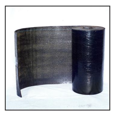
MIGHTYPLATE MODIFIED BITUMEN FLASHING MATERIAL is made with the same material as MIGHTYPLATE MODIFIED BITUMEN ROOFING MEMBRANE. It is cut to 18" by 32'9" to make roof flashing and detail work convenient to accomplish.
