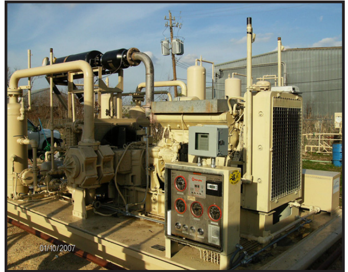
Typical applications for L. P. & NATURAL GAS ENGINE OIL are stationary engines, burning either natural gas or l.p. gas, which call for low-ash-type oil.
