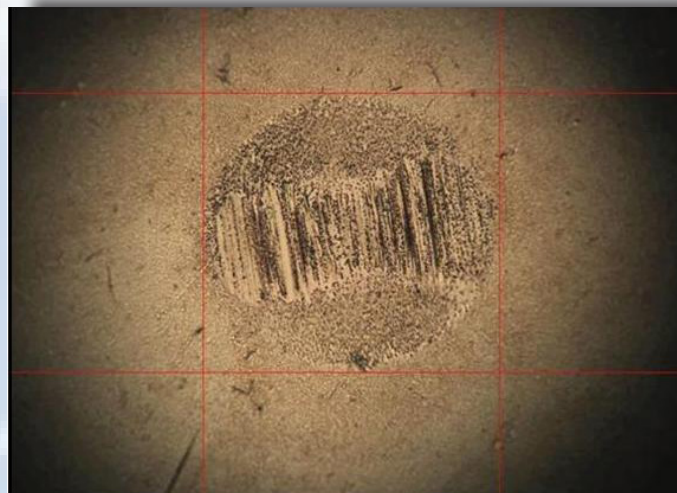
This wear scar is a perfect example of how low lubricity in fuel can damage fuel system components.
